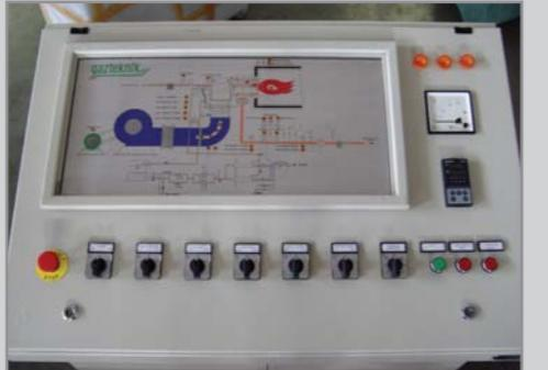
The table type control panel is made of steel. This panel includes program relay, contactors for combustion air fan, relays fuses, signal lamps and all the wiring connections are finished.
