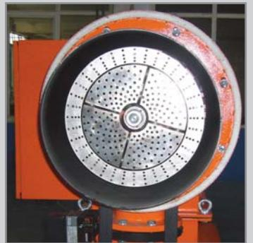
ECOSTAR COMBUSTION SYSTEM provides different type of mixing unit boilers. Because we adjust flame dimension according to the combustion size this is the most advantage of ECOSTAR COMBUSTION SYSTEM burner. Because of adjustable gas nozzles also provides capacity change and formation of flame.
